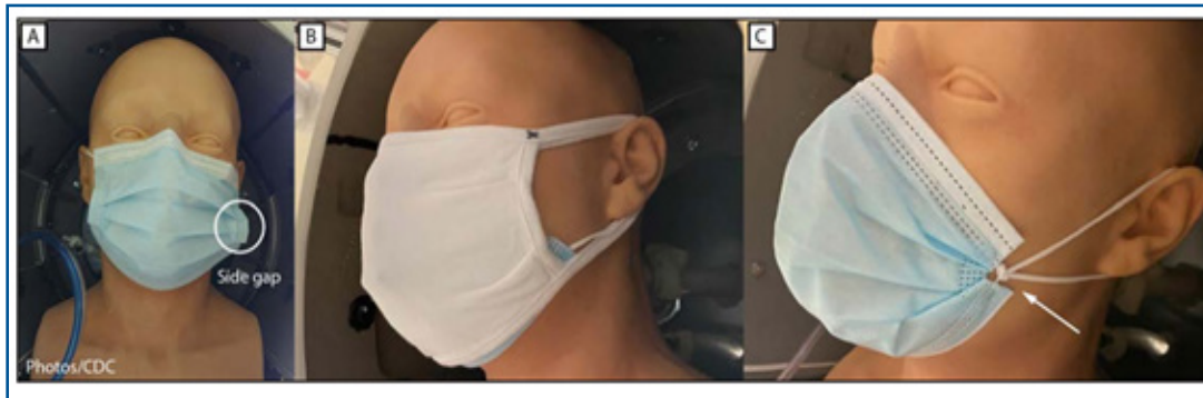
Figure 1: Tested masks, including A, knotless medical procedure mask; B, double mask (tissue mask covering the medical procedure mask); and C, knotted / folded medical procedure mask. Figure extracted from the original article of the Center for Disease Prevention and Control in the United States 11 .
